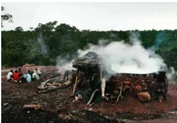
A brine well supplying sites on both river shores (1), Evaporation of the brine in salt kilns (2, 3) (Kigoma, 2018 – Photo: IPIS)
