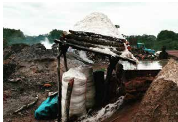
A brine well supplying sites on both river shores (1), Evaporation of the brine in salt kilns (2, 3) (Kigoma, 2018 – Photo: IPIS)
