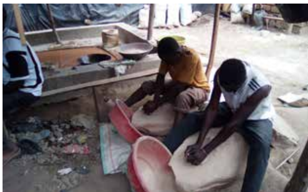
In the absence of a ball mill miners grind the ore manually (1), Foreign investment on a PML (2) (Mara, 2017, Photo: IPIS)
